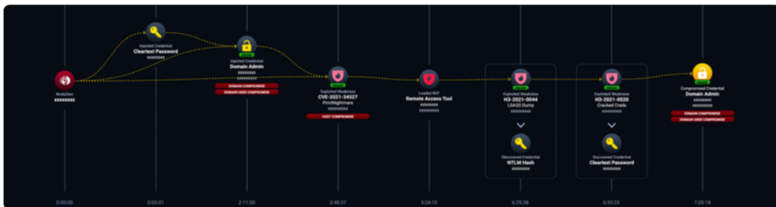
▲ Figure 5 Attack path showing host, domain admin, and domain compromise using an injected cleartext password and the NodeZero RAT.
