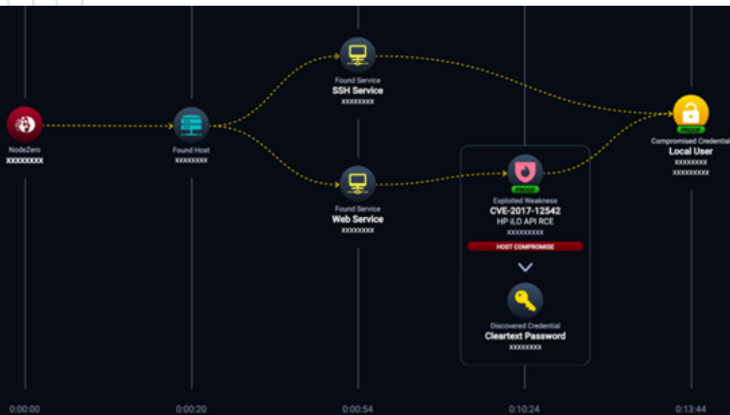
▲ Figure 9 Attack path shows NodeZero leveraging CVE-2017-12542 and discover local admin cleartext password leading to host compromise.
